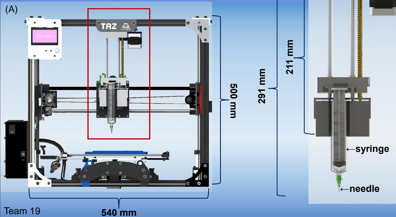
Figure 10. (A) The full 3D printer system after retrofitting the syringe pump. (B) A blow up of the syringe assembly with major parts labeled.
