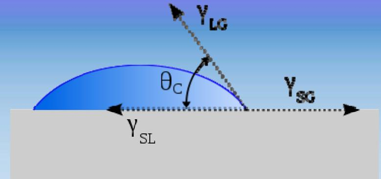
Figure 3. A liquid droplet on a substrate with interface angle labeled.
