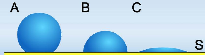
Figure 4. An example of varying droplet geometries and their contact angles with surface S; (A) large contact angle; (B) medium contact angle; (C) small contact angle
