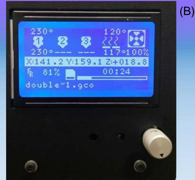
Figure 12. (A) Webcam with gooseneck clamp. (B) Control interface on printer with a print in progress.
