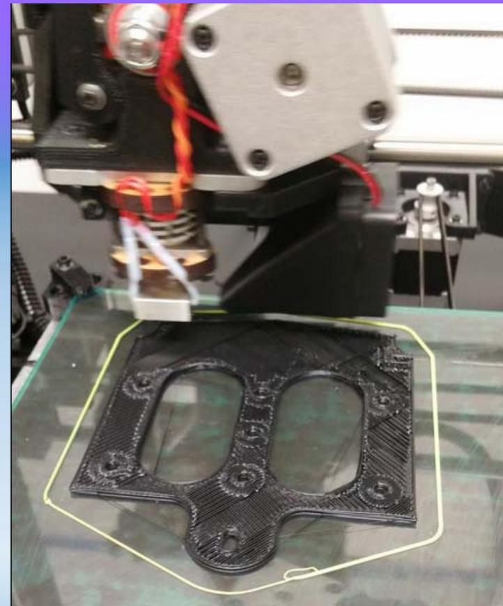
*Figure 11. Printing part of the mount for the syringe to be retrofitted onto the existing printer.*
