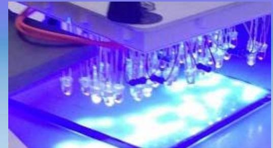
*Figure 8. Testing the polymer curing time with UV LED bulbs.*
